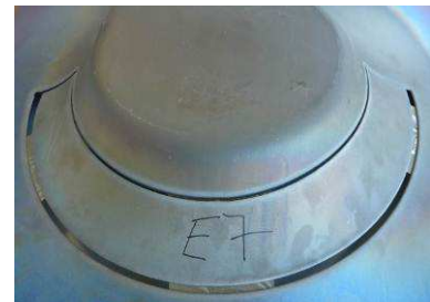
Hot formed Ti 6Al-4V shape shows low distortion after trimming
